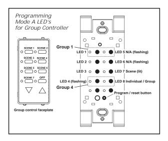
Step 2: Quickly press (2 seconds) and release the programming button to place Group Controller in Programming Mode A. This mode is confirmed when the 8 LED's are lit or flashing.
